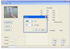
Switch on the SUR, then launch SURsoft, and begin communication with the SUR by selecting the Connect command from the File menu of SURsoft:
