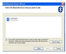
The SUR is now 'discovered', which leads to the next step, pairing. This step involves establishing a unique relationship between the host PC and the Bluetooth device, exchanging a 'passkey' to allow error free communication between these devices. Unless otherwise specified, all SUR-3BT units have a passkey of "1234", and is provided in the next step by highlighting the SUR device, clicking "Next", and filling in the subsequent screen:
