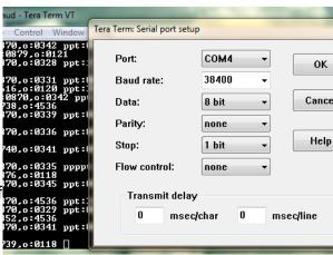
The RovR communicates via its serial port with parameters fixed at 38.4K baud, 8 bit, and no parity.
